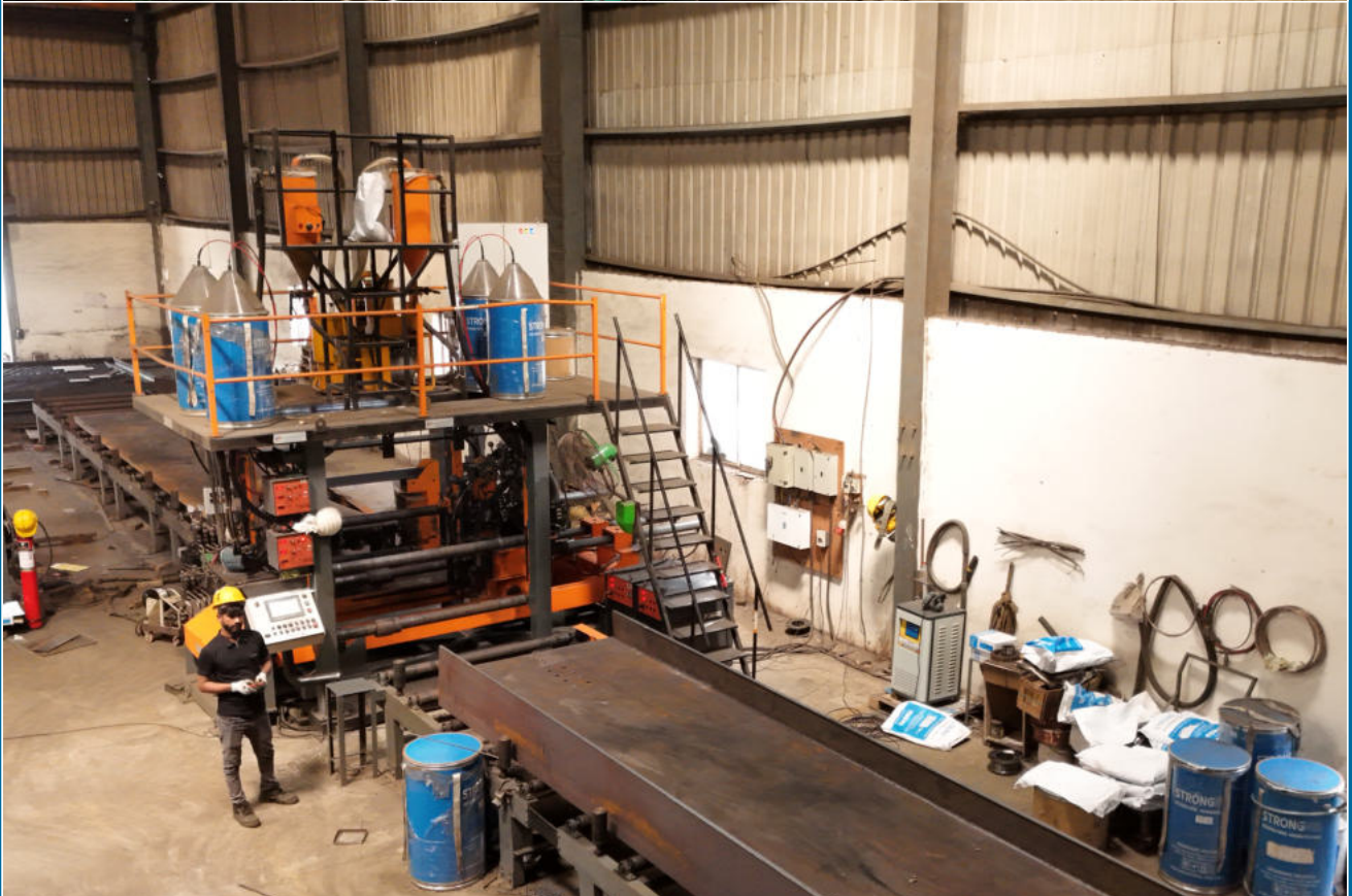
H BEAM PTW WELDING MACHINE NO.1 & MACHINE NO. 2
