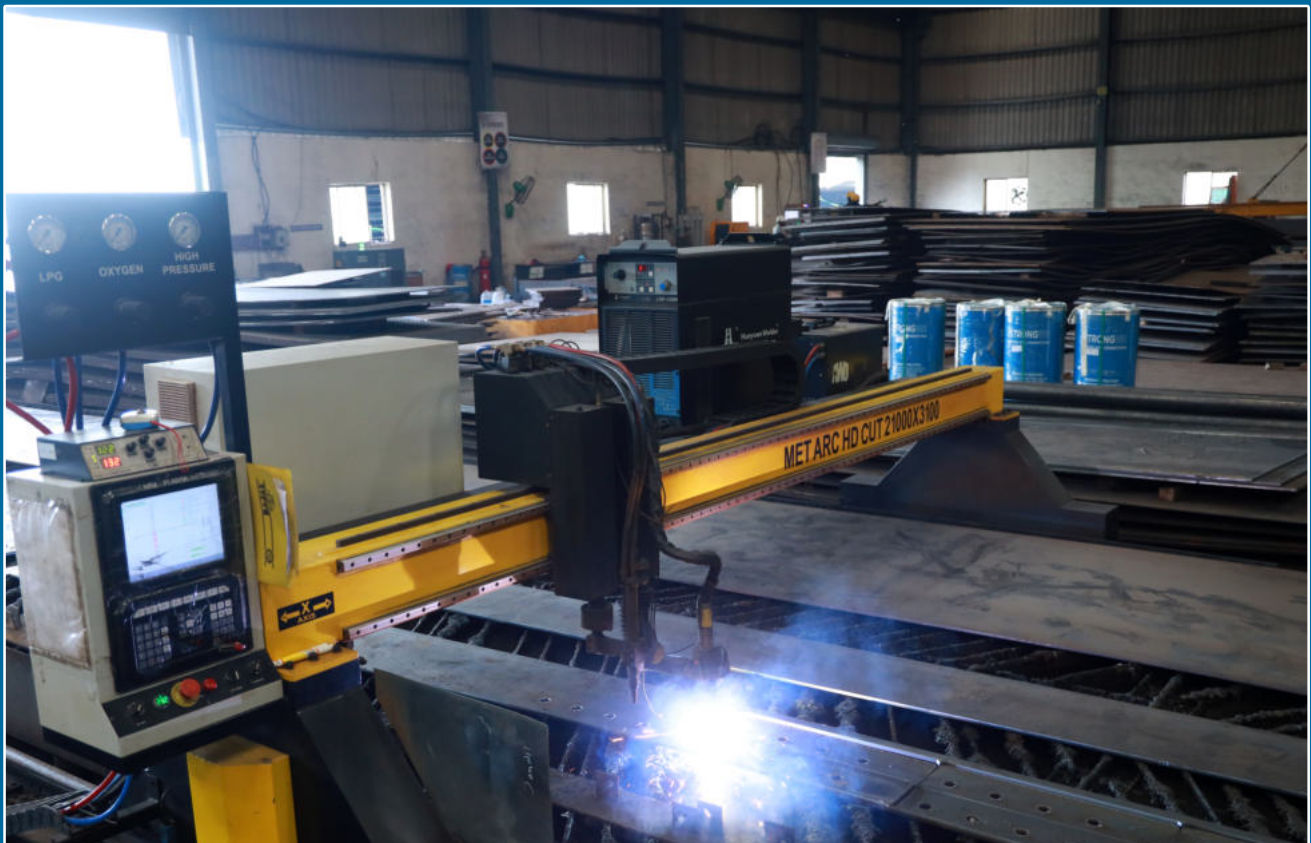
OXY & FUEL CNC PLASMA CUTTING MACHINE NO. 1 (24 MTR X 4.2 MTR)
