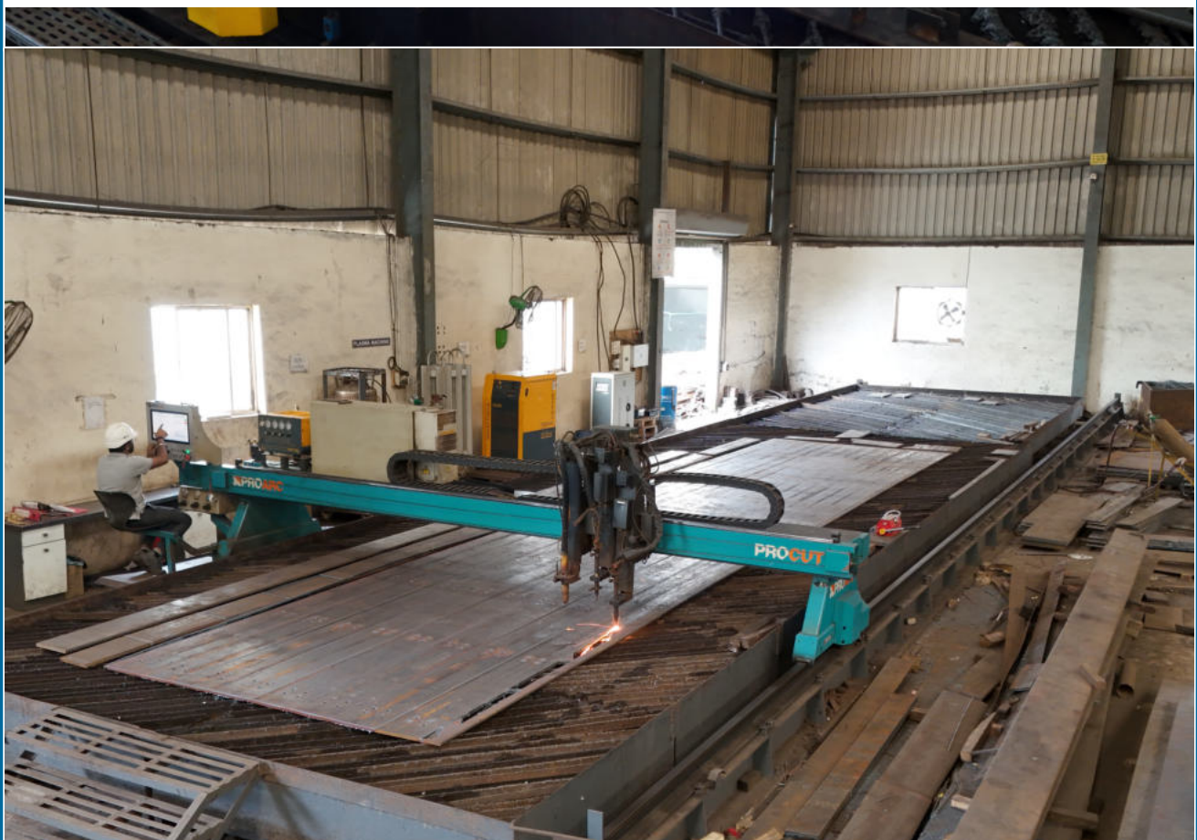
OXY & FUEL CNC PLASMA CUTTING MACHINE NO. 2 (24 MTR X 4.2 MTR)
