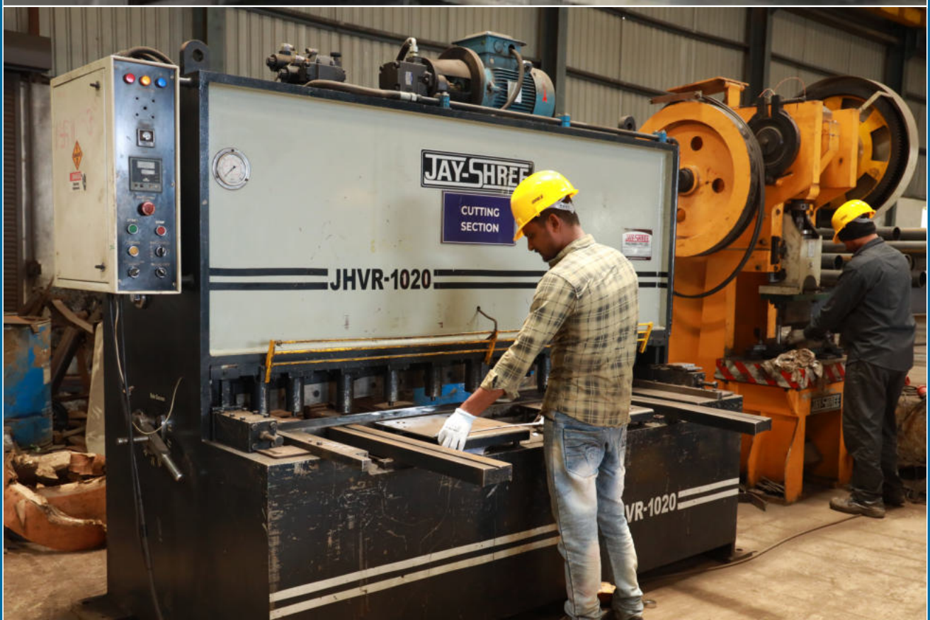
HYDRAULIC SHEARING MACHINE 16MM THICKNESS CUTTING
